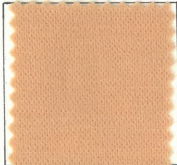
3. Crossmiss interlock (RWCS wool yarn)
