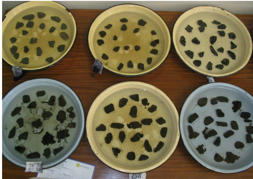
Figure 1: Samples D1 to D3 (top row) and D7 to D9 (bottom row) after soaking in glycol for 45 days
