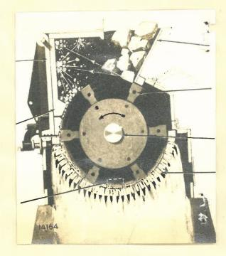
are all of the same size and the number of bars in each panel vary inversely with the clear opening between them. The manufacturer's ratings for this machine are as follows: Diameter of outer circle of hammer travel = 15" Width of rotor = 8" Approximate horse power = 7 - 8 Speed in r.pm. = 1800-3000  $1^{1''}$ Capacity (8 bar opening) =  $\frac{3}{4}$  - 1 ton/hour. Capacity (1" bar opening) = 2 - 3 ton/hr.
