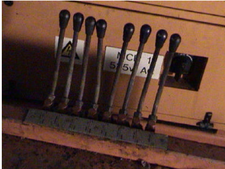
Figure 1.32: Awkward layout of the control levers
