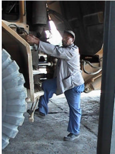
Figure 1.7: Three-point contact for easy access
