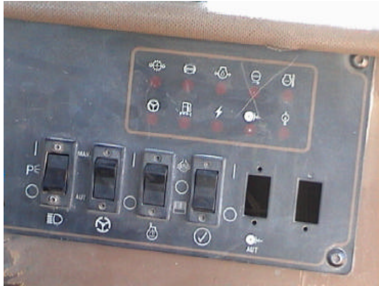
Figure 1.12: Symbols used for labelling the controls
