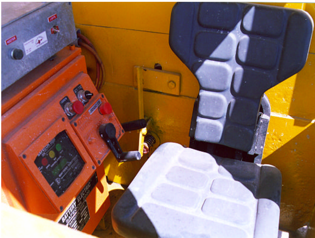
Figure 3.2.4: Seat with T-shaped backrest
