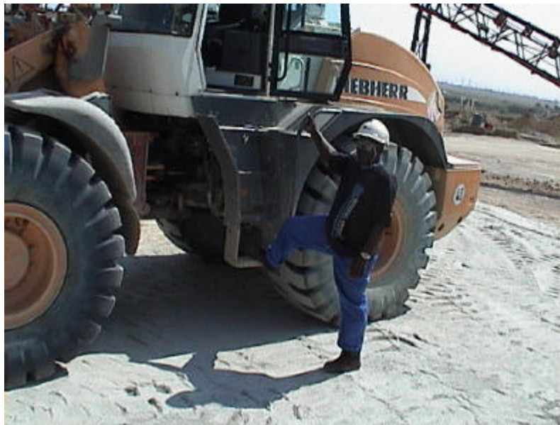
Figure 1.23: Three-point contact for easy access
