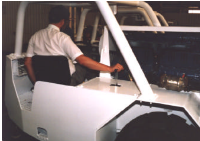
Figure 1.36: Awkward location of the control lever
