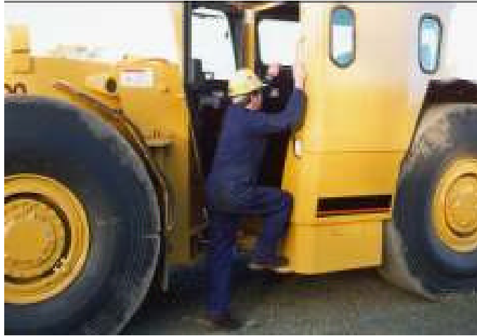
Figure 1.18: Three-point contact for easy access
