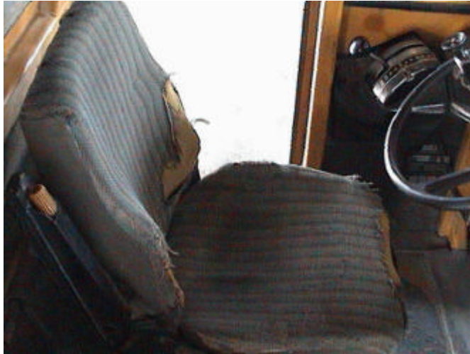
Figure 1.8: Unsuitable seat fabric for mining machinery
