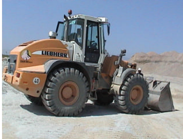
Figure 1.26: Improved visibility around the cab
