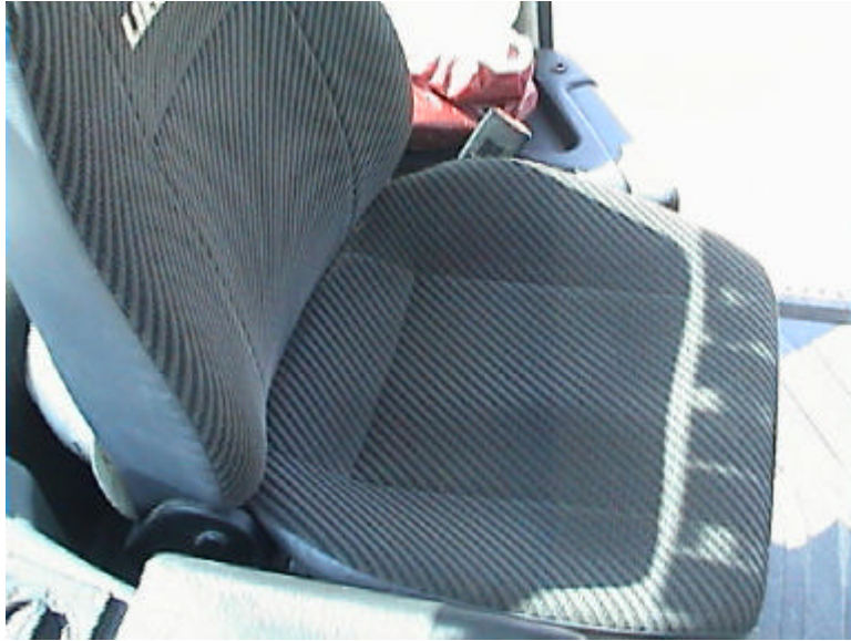
Figure 1.24: Unsuitable seat fabric for a mining vehicle
