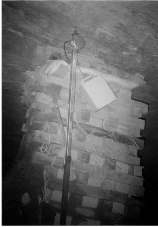
Figure 26. A potentiometer closure meter integrated with a spring-loaded telescopic tube. Note the external logger used to collect the data.
