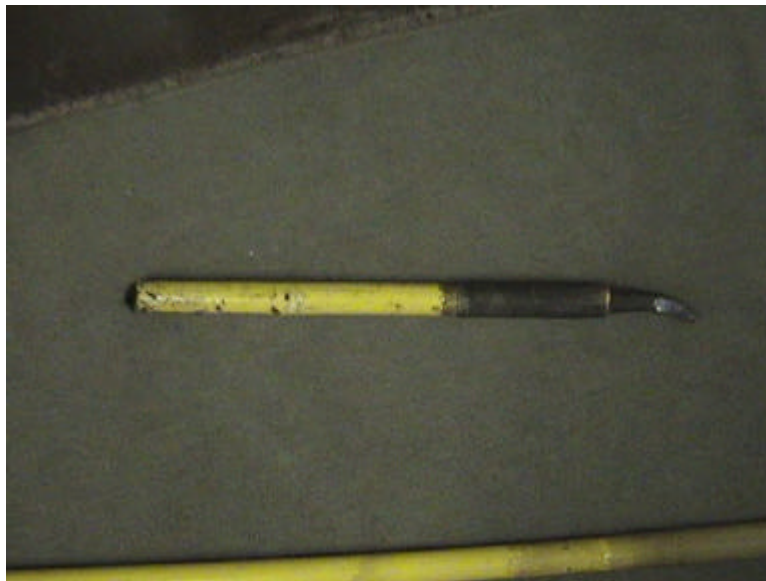
Figure 3-15: Damaged pinch bar.
