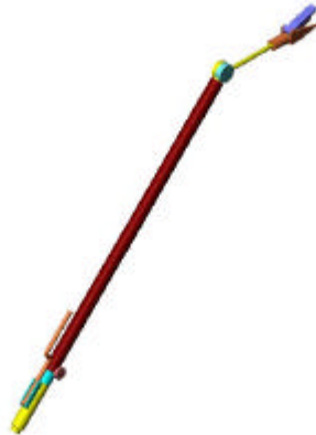
Figure 4-9: Solid model of prototype mechanical “jaws”.
