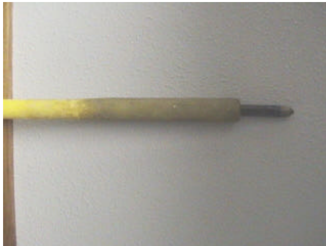
Figure 3-5: XDM lightweight pinch bar with extruded glass fibre tube.
