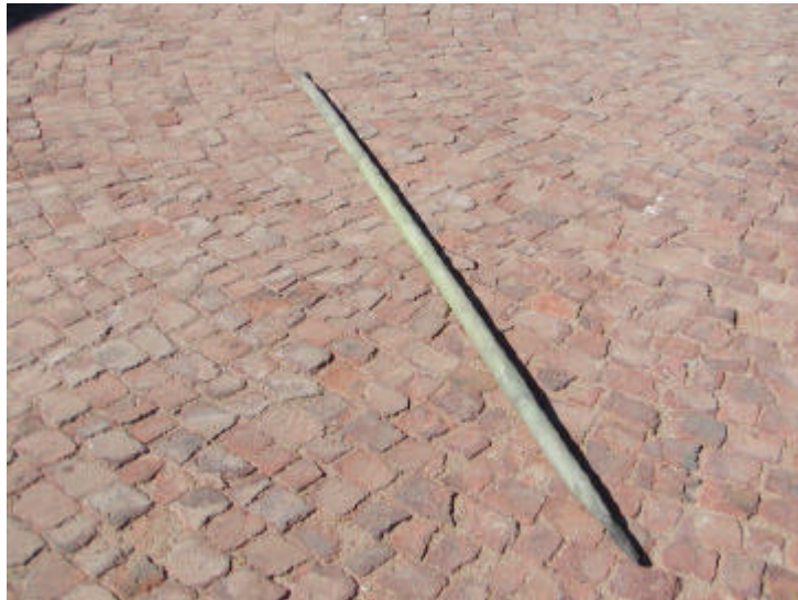
Figure 3-4: XDM lightweight pinch bar with manufactured glass fibre bar.
