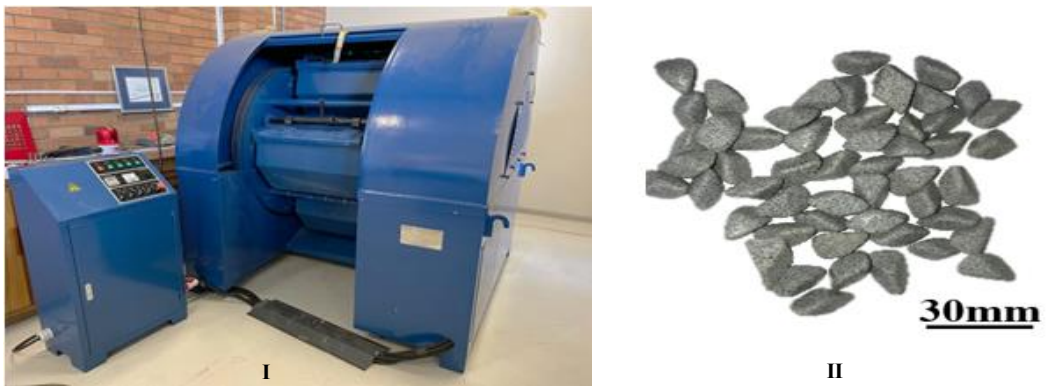
Figure 2. CB320-CBF Machine (I) and ceramic media (II)
