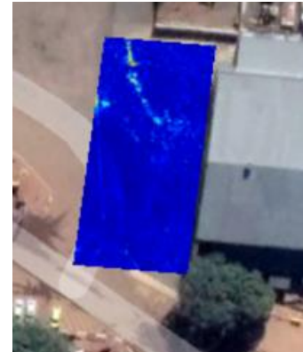
Figure 5. Georeferenced GPR depth slice overlain on a Google Earth image
