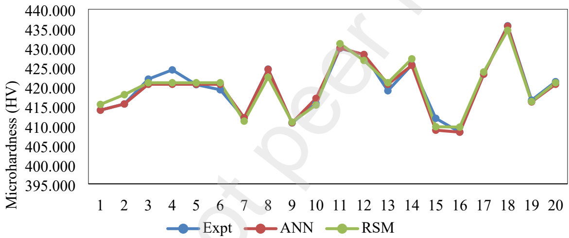
Figure 21 Comparison of experimental outcomes with ANN and RSM models results on microhardness
