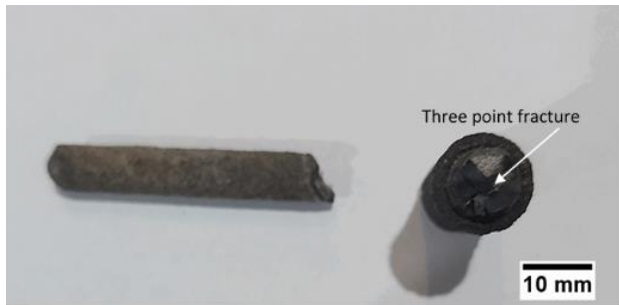
Fig. 10. Fracture surface of LENS® fabricated rotary burr
