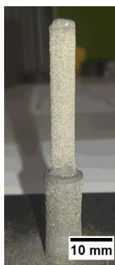
Fig. 7. LENS® fabrication of a cylindrical rotary burr with preheat of 250°C
