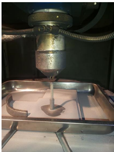
Fig. 6. LENS fabrication of the cylindrical rotary burr
