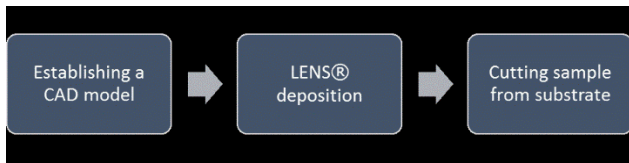
Fig. 4. LENS® process flow for the manufacture of the prototype burr
