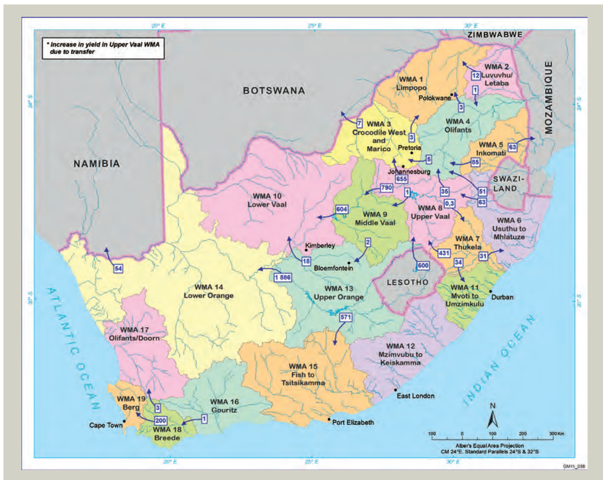
Figure 1.5 Location of Water Management Areas and major inter-WMA transfers. The figures on each arrow are in Mm 3 per year for the scheme [7].
