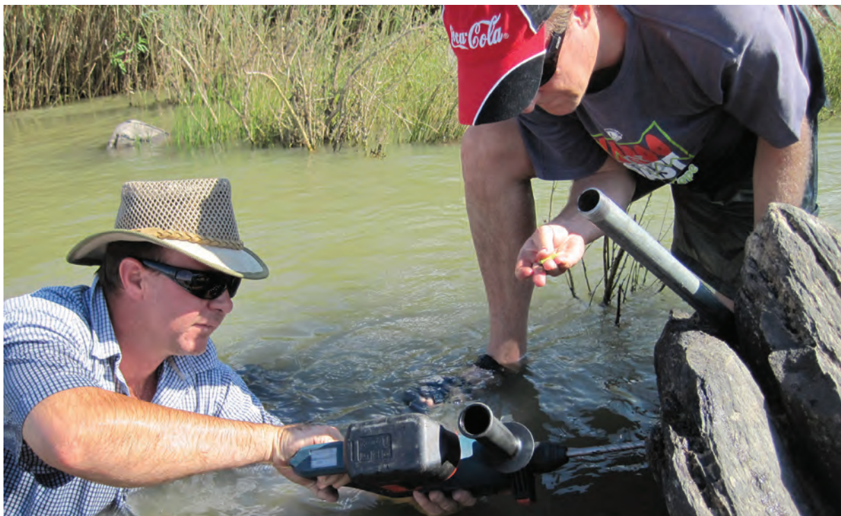
James MacKenzie and Drew Birkhead installing a data logger in the Orange River downstream of Boegoeberg Dam to measure water levels for use in hydraulic modelling as part of the EWR determination, March 2010.
