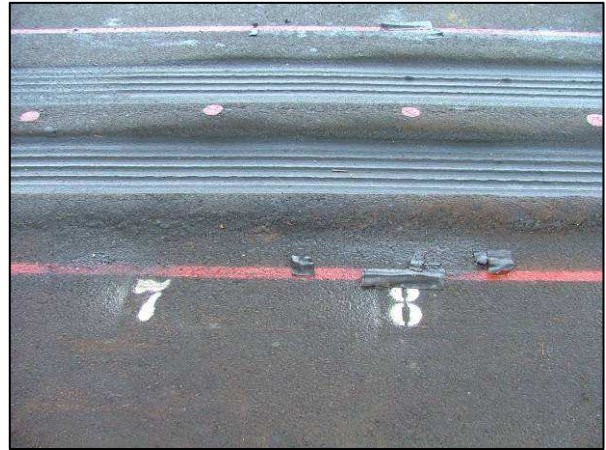
(b) Heavy Vehicle Simulator test section on R80 outside Pretoria (tested at an equivalent 80 kN axle load at 60°C)
