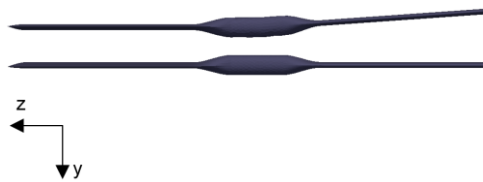
Fig. 7. Healthy and faulty blade model showing offset blade.
