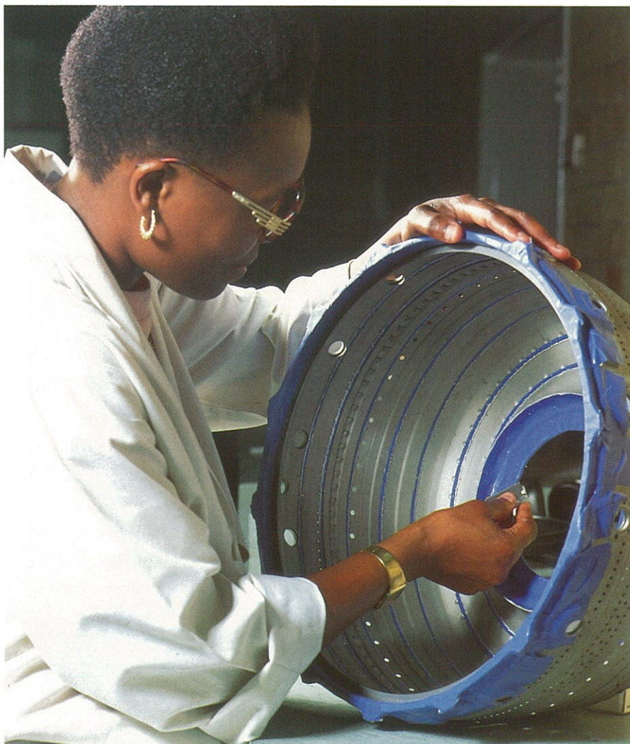
Masking of a gas turbine combustion chamber before applying a plasma sprayed ceramic coating.
