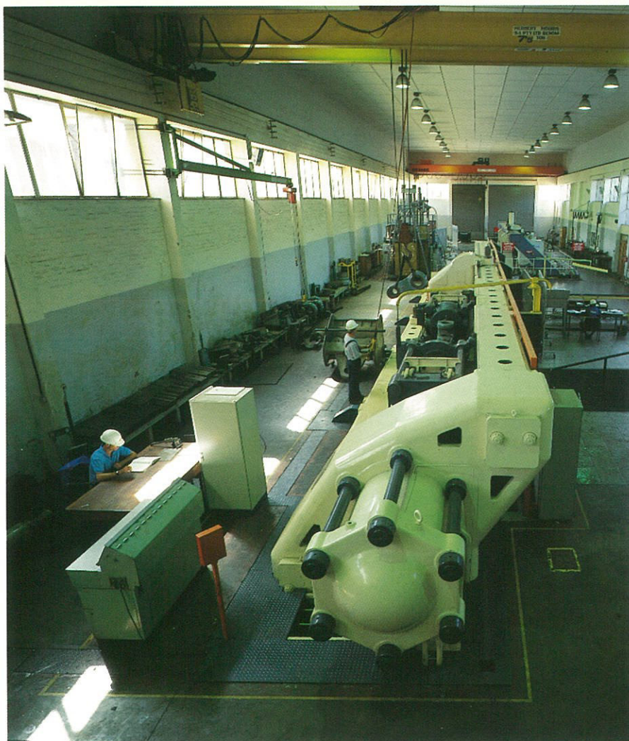
The CSIR's mine rope testing facility at Cottesloe, Johannesburg.
