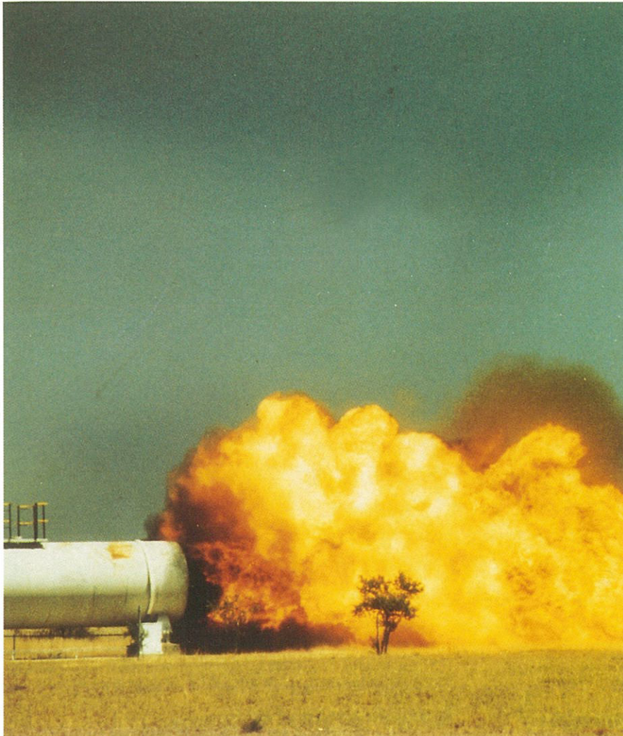
The mild steel tunnel for research into coal dust explosions at the CSIR's Kloppersbos explosion research facility near Pretoria which is part of Miningtek.
