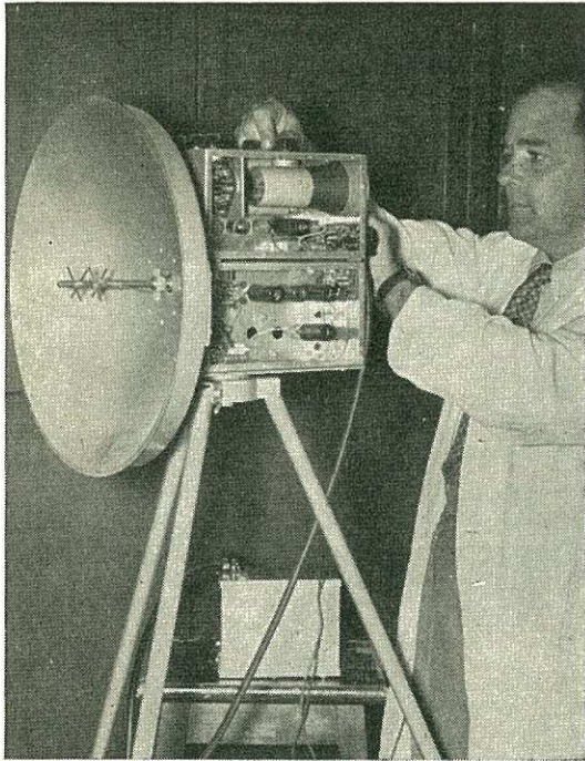
Mikrogolfoerusting deur die T.N.L. ontwikkel vir afstandsmeting. Microwave equipment developed by the T.R.L. for distance measurement.
