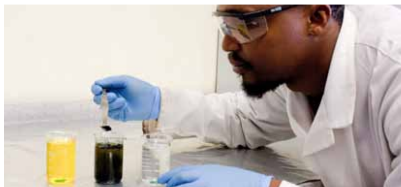
PhD student Katlego Setshedi adds clay nanocomposites to a wastewater sample polluted with chromium (VI). Once the yellow polluted water has been passed through the nanoclay composite the effluent is clear and clean, as seen in the transparent water sample.
