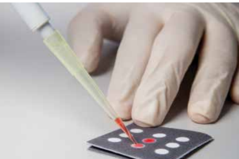
A pipette is used to spot reagents onto a wax-patterned paper diagnostic device.
