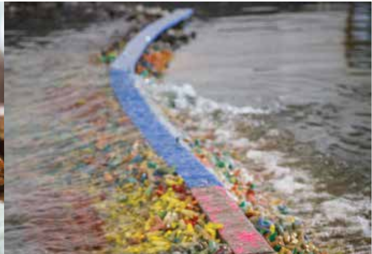
The scaled physical models of harbours and breakwaters built at the CSIR coastal laboratory are constructed in fine detail and with great care to ensure utmost accuracy.
