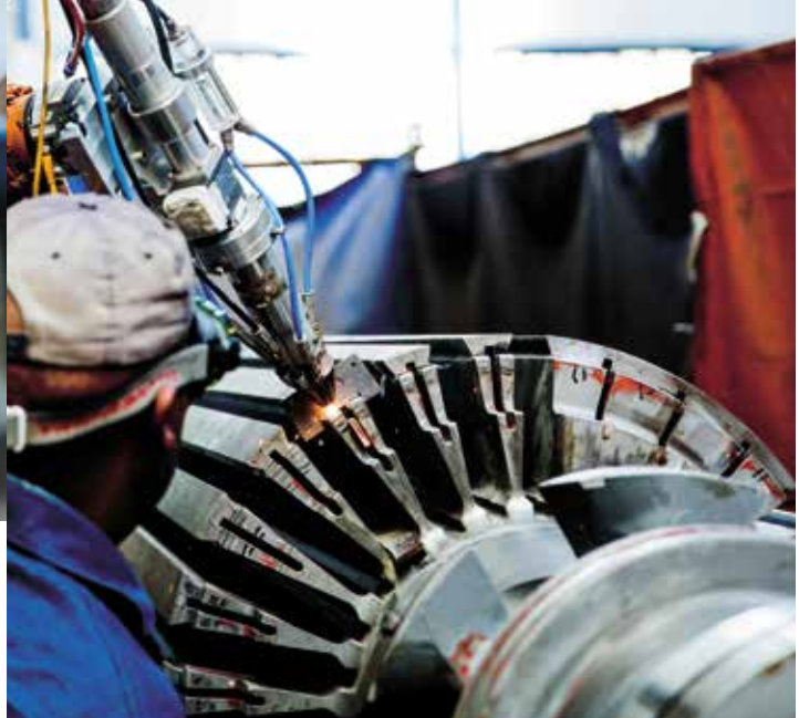
Above and right: A mobile laser-based refurbishment system designed and constructed by CSIR engineers. The system can repair high-value components on-site and reduce metallurgical damage on an extended heat-affected zone while offering quick turnaround times.
