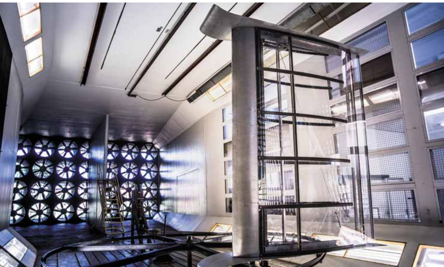
The transparent wing of a new turbine is being tested in the CSIR's seven-metre wind tunnel for its South African inventor.
