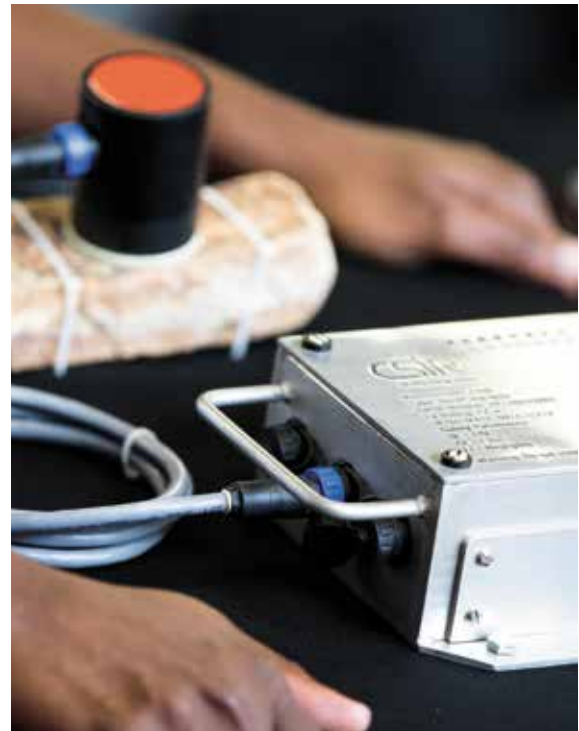
A CSIR-developed microseismic data acquisition and processing platform serves as an early-warning system for large rockfalls and helps optimise safe re-entry time after blasting operations.
