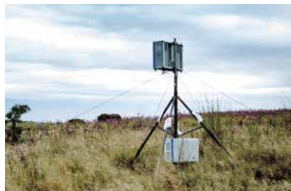
The multistatic radar technology deployed at the Rietvlei Nature Reserve in Pretoria for field tests. The system can detect and localise micro-drones at ranges of up to a few kilometres. It is designed to look throughout the entire surveillance area to enable rapid warnings of potential drones and fine tracking of their movements.
