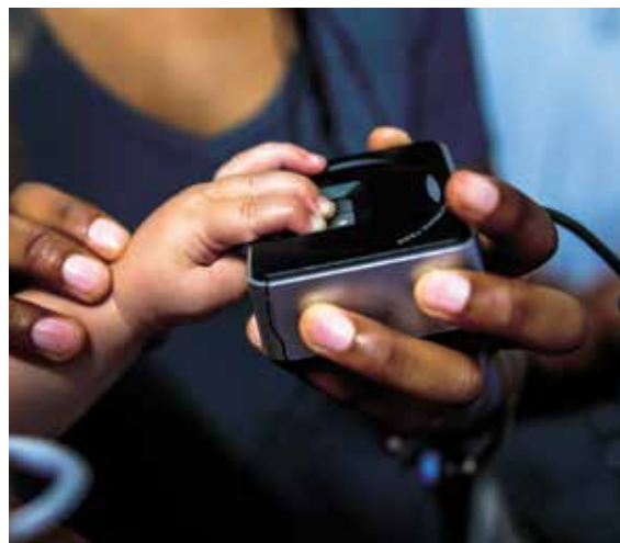
The CSIR has developed a biometric recognition system to capture clear fingerprints of infants.
