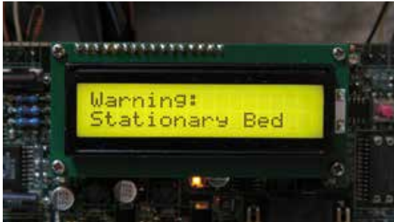
The CSIR-developed instrument has detected particle deposits at the bottom of a slurry pipeline and issues a warning.
