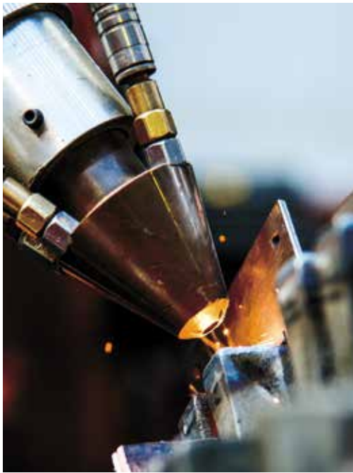
Above and right: A mobile laser-based refurbishment system designed and constructed by CSIR engineers. The system can repair high-value components on-site and reduce metallurgical damage on an extended heat-affected zone while offering quick turnaround times.
