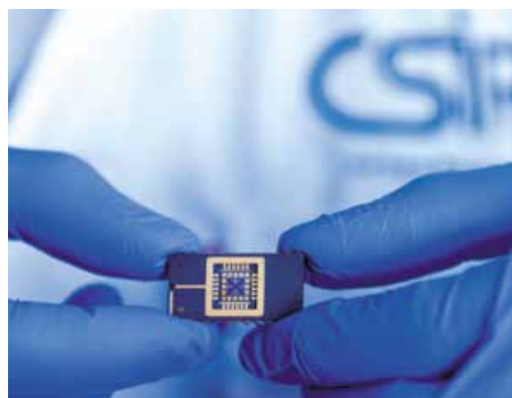
An eight-transistor microchip containing nanoparticles with electronic properties that are used to tune-in to specific gases.
