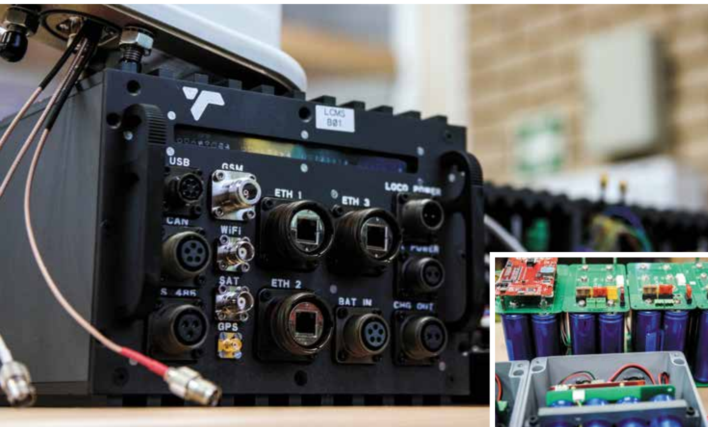
Above: The locomotive condition monitoring system in a ruggedised enclosure with the roof-mounted antenna. (Right) The system's integrated battery backup system.
