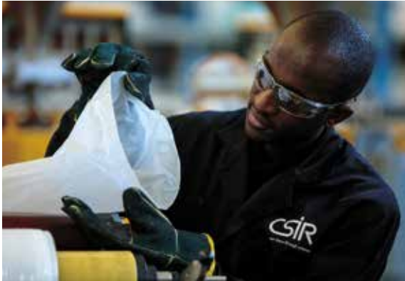
The CSIR has developed technology for biodegradable plastic. Researchers use biopolymers and agricultural biomass by-products for flexible film packaging such as plastic carrier bags and food wrapping. Technologist Sifiso Skosana inspects a bag produced at the CSIR.
