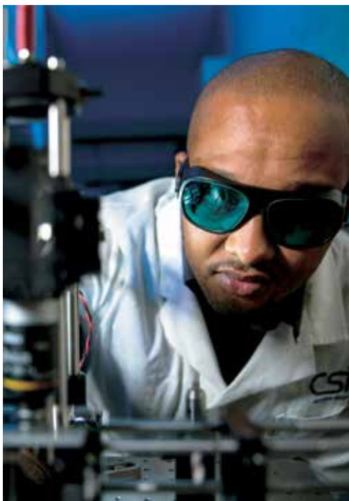
CSIR senior researcher Dr Sello Manoto with an in-house built reflectance spectroscopy platform for HIV detection and viral load quantification.
