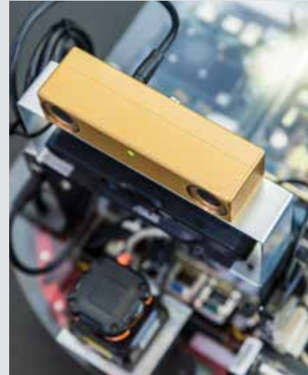
Key features of the robot include a stereo-vision camera (the gold coloured sensor at the top) for 3D imaging, and a low-power, mobile graphics processing unit (mounted at the back of the robot) for real-time image analysis.
