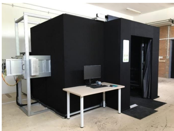
Figure 5: A+A+A+ Sun simulator with integrated thermal chamber at CSIR campus Pretoria
