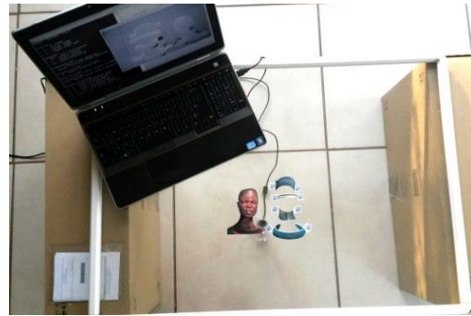
Figure 6: Setup showing the computer, camera, clear construction surface with a white frame, and supports.
