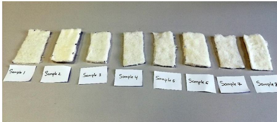
Figure 5: Samples of CFF:BCF nonwoven fabrics produced at different run
