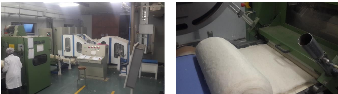
Figure 3: Machines used for needle-punched fabrics (on the left); CFF:BCF nonwoven fabrics leaving the needle puncher (on the right)
