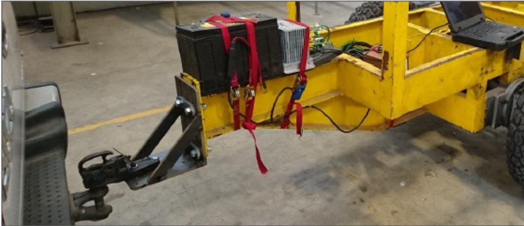
**Figure 6: Adjustable tow hitch**
