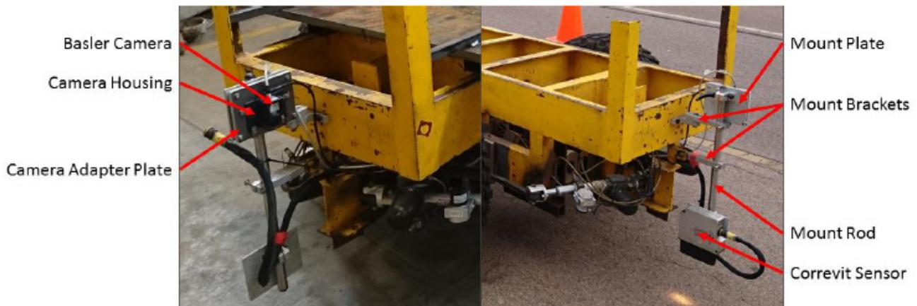
**Figure 5: Correvit Sensor and Camera bracket**
