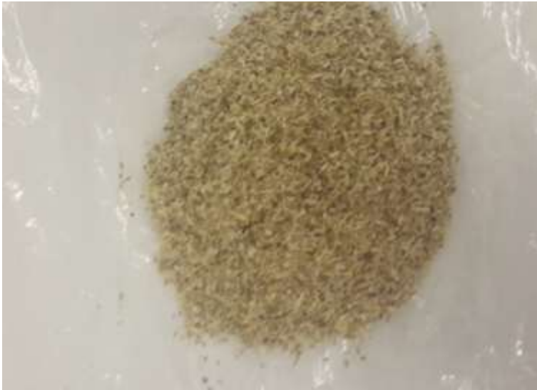
Figure 220: Close-up of the dired and milled sample of soya bean field residues
