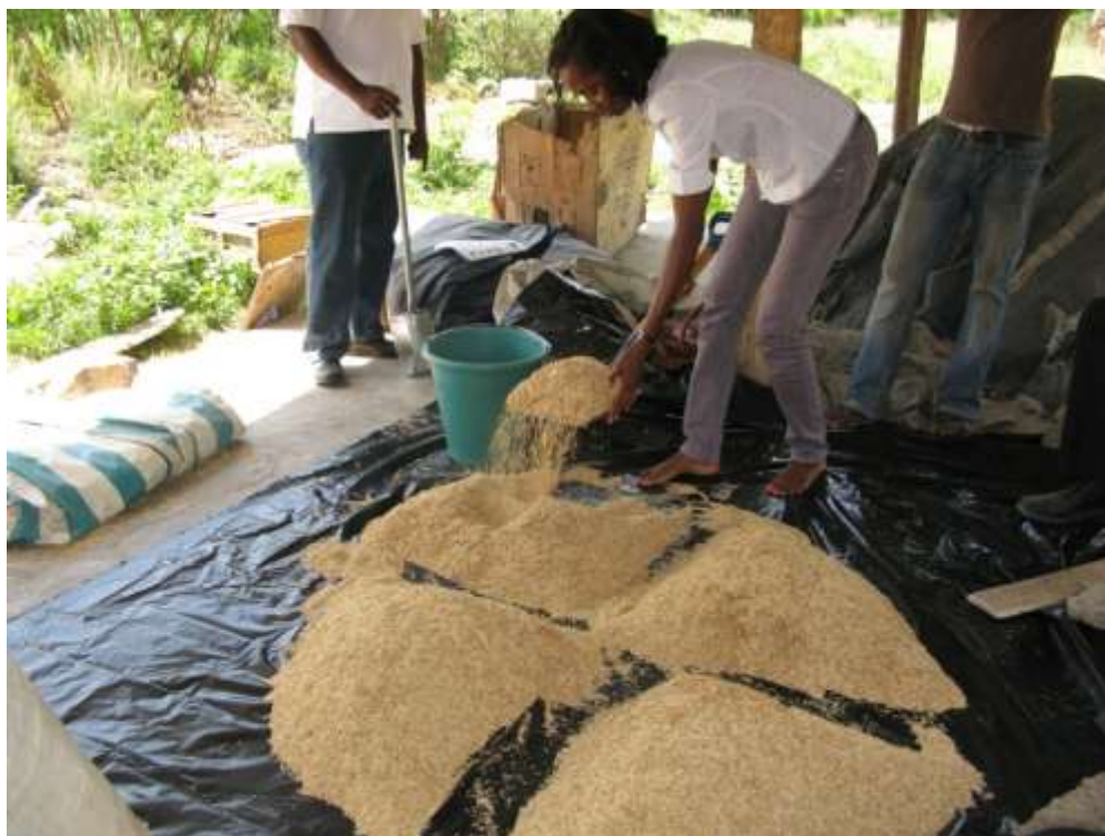
Figure 4: Coning and quartering in progress as part of the process of creating a final sample. The biomass here is rice husk.
