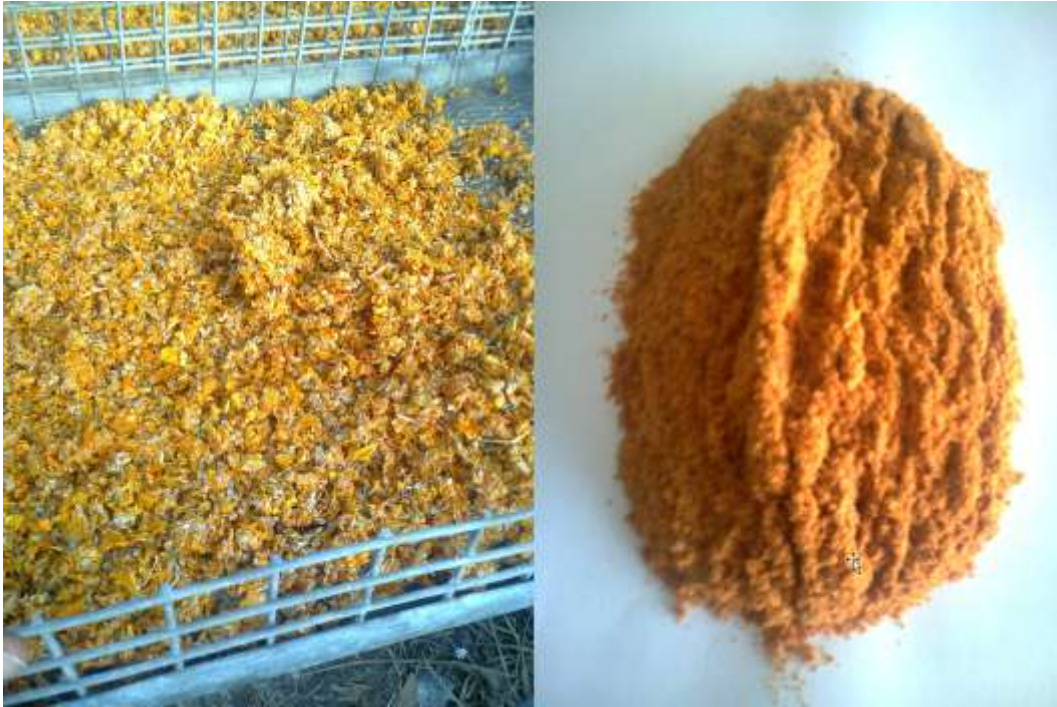
Figure 197: The untreated tomato pulp waste (to the left), dried and milled sample of tomato pulp (to the right)
