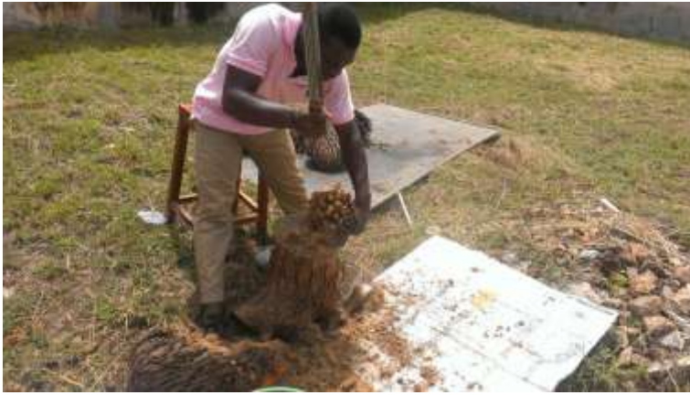
Figure 75: Size reduction of the sampled empty fruit bunches before drying.
