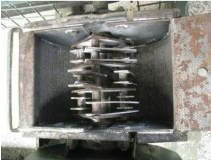
Figure 106: The inner part of the hammer mill used for milling
