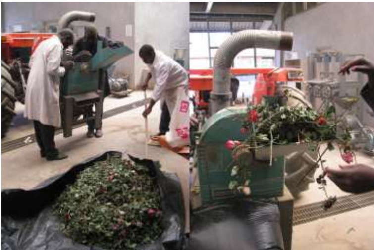
Figure 124: Milling of flowers in tractor driven hammer mill
