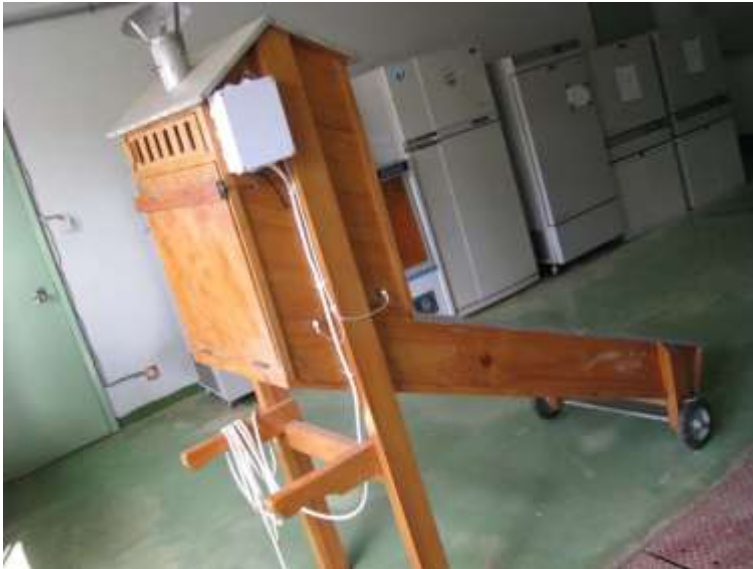
Figure 158: A pilot plant solar dryer equipped with an electric heating coil to supplement solar energy
