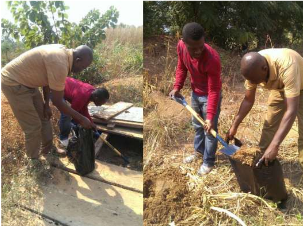
Figure 79: Sampling in progress. To the left sampling from collection pit and to the right collection from heap
