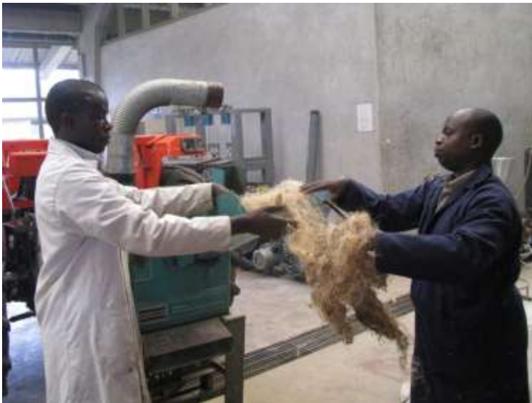
Figure 154: Milling the sisal processing biowaste with a hammer mill
