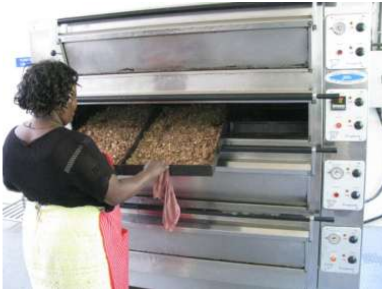
Figure 103: Oven drying of cassava chips at the Food Science Workshop, JKUAT
