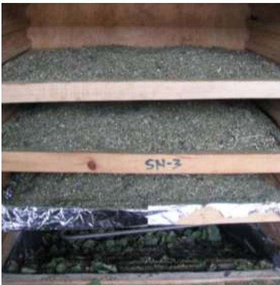
Figure 125: Solar drying of milled flowers, this also constitutes the form of the final sample
