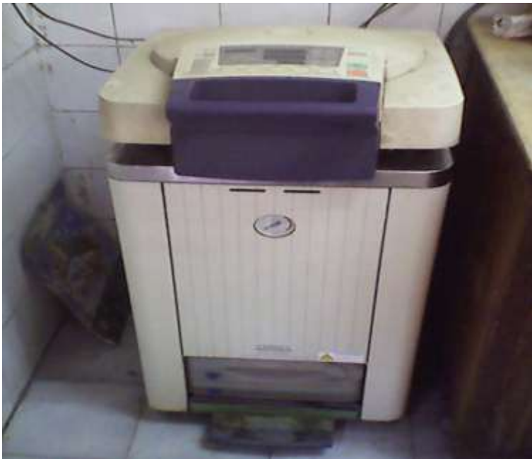
Figure 33: Autoclave used in the analysis of the sample
