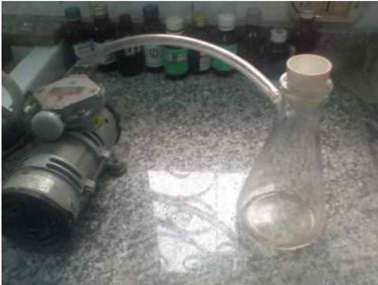
Figure 19: Filtration system, equipped with a vacuum pump connected to, by plastic hose, a Büchner flask that is fitted with a Gooch crucible.
