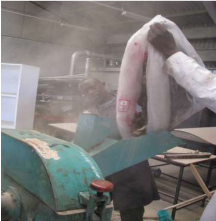
Figure 133: Milling of the sample using a tractor driven hammer mill
