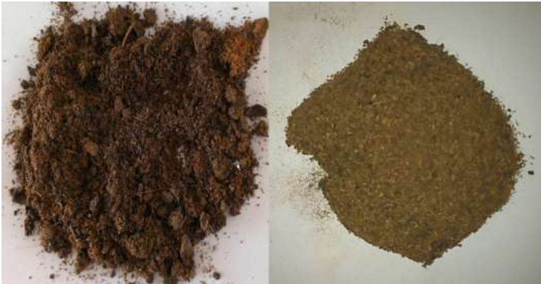
Figure 80: Close-up of untreated sample of pig manure (to the right) and dried and milled sample of pig manure (to the left).
