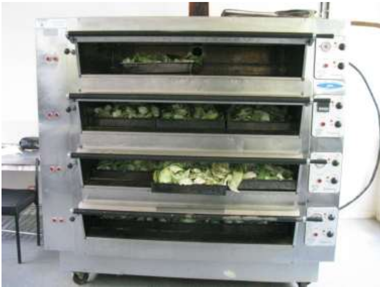
Figure 93: Oven drying of cabbages at department of Food Science and Technology Workshops, Kenya
