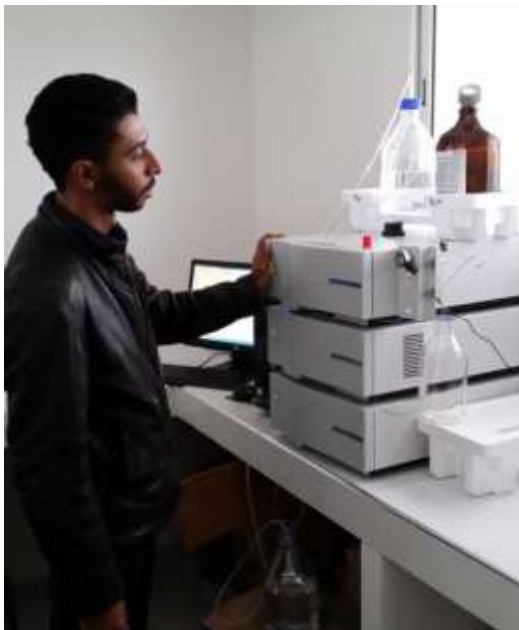
Figure 183: HPLC system used for strong acid hydrolysis
