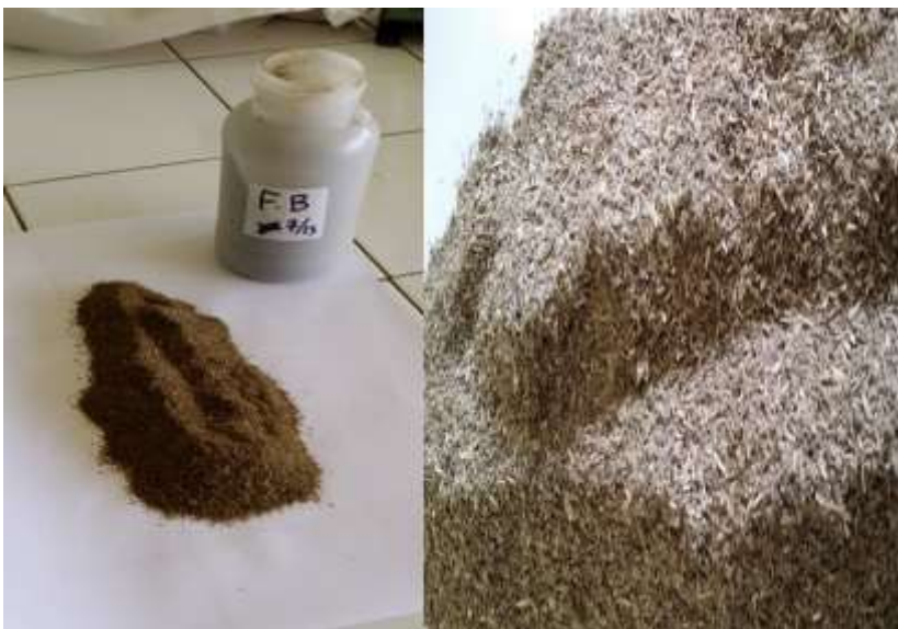
Figure 179: Dried and milled sample of cattle manure (close-up of final sample to the right)
