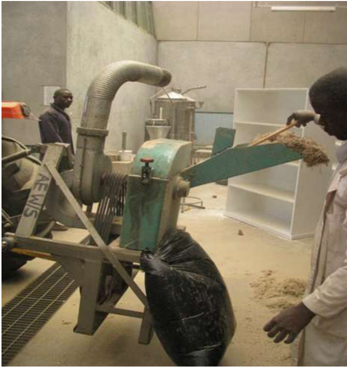
Figure 160: Bagasse milling using a tractor driven hammer mill
