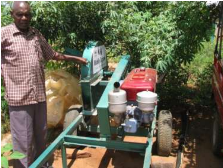
Figure 101: A mobile chipper used for size reduction of the cassava waste materials
