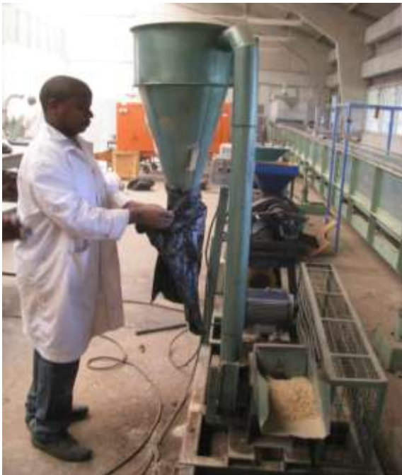
Figure 112: Milling of coffee husks using a hammer mill
