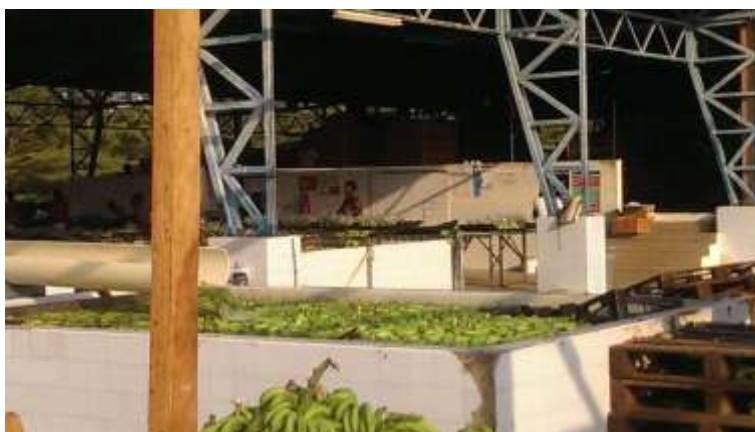
Figure 46: Water is used to clean and transport the rejected banana
