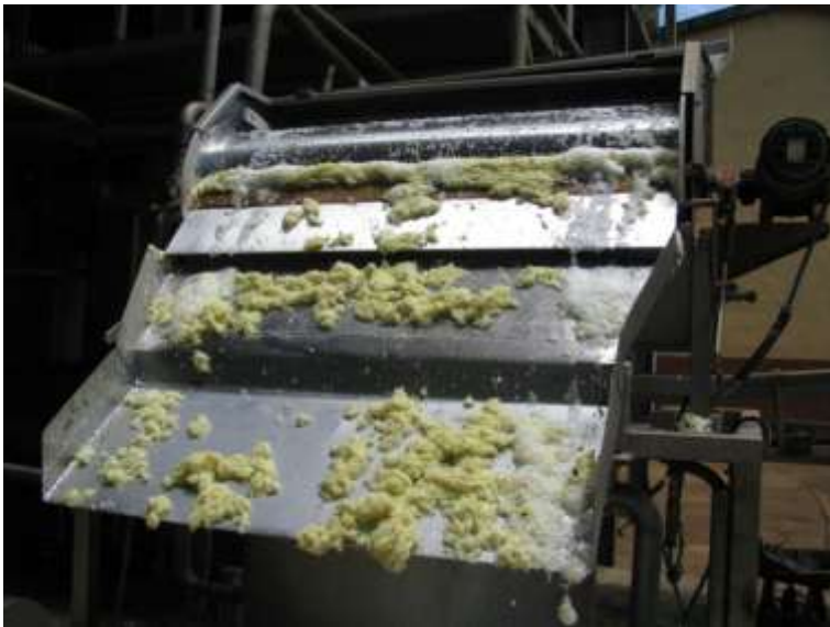
Figure 137: Pineapple core coming out after the press
