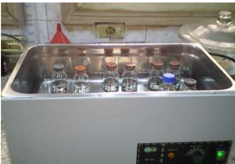
Figure 32: Water bath used in the analysis of the samples
