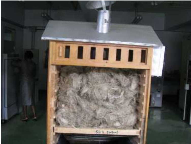
Figure 153: Drying of sisal waste in an electric assisted solar dryer (70°C)
