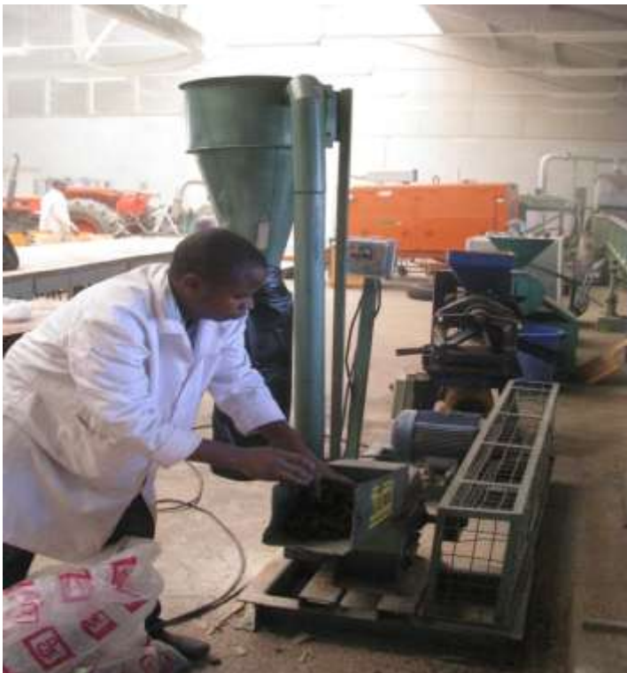
Figure 94: Milling of dried cabbage waste using a hammer mill
