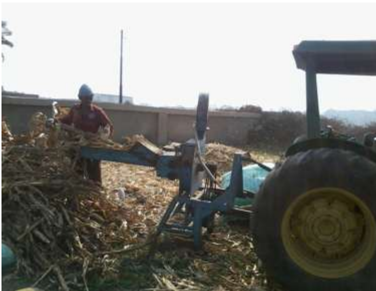
Figure 17: Chopping of corn stover, tractor used to power the equipment
