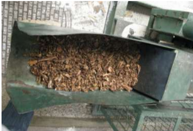
Figure 104: Close-up of sample in the feed hopper of the mill
