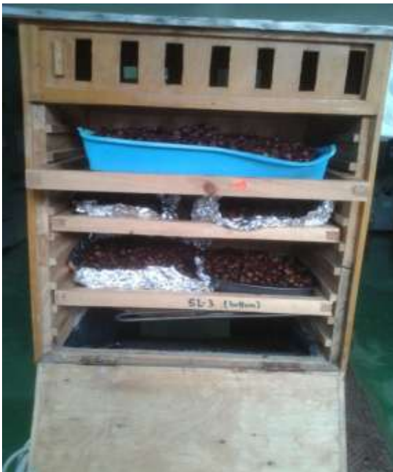
Figure 115: Drying coffee pulp in a solar dryer at 70°C
