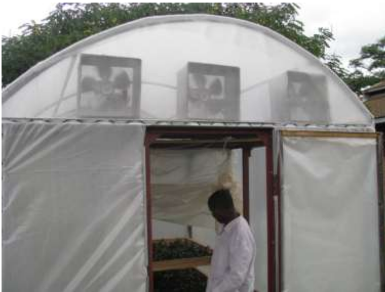
Figure 122: Greenhouse solar dryer used for predrying of flours (temperature 45-50°C at peak hours)
