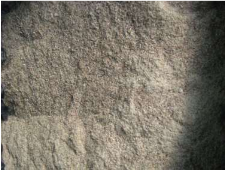
Figure 142: Dried and milled final sample of mixed core and peels pineapple processing waste
