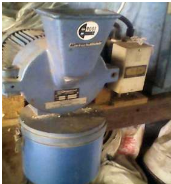
Figure 38: Milling machine used for milling the samples Egypt
