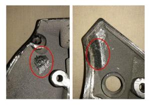
Figure 11: Areas with difficult support removal
