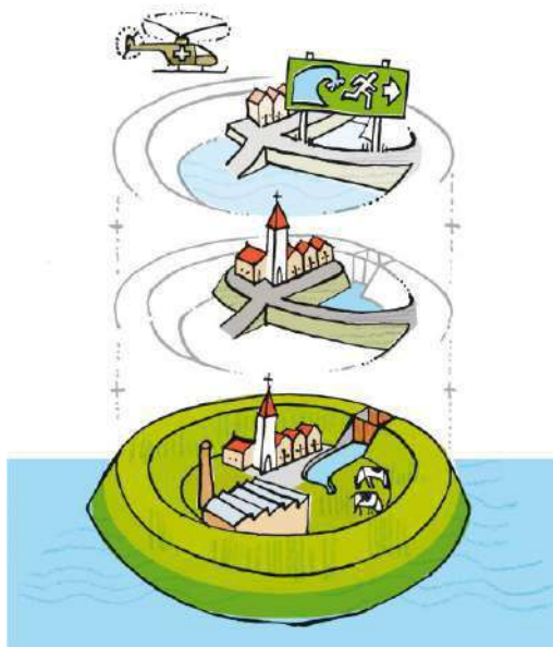
Figure 3: Multi-layer safety; prevention, sustainable spatial planning and disaster management . Source: Government of the Netherlands
