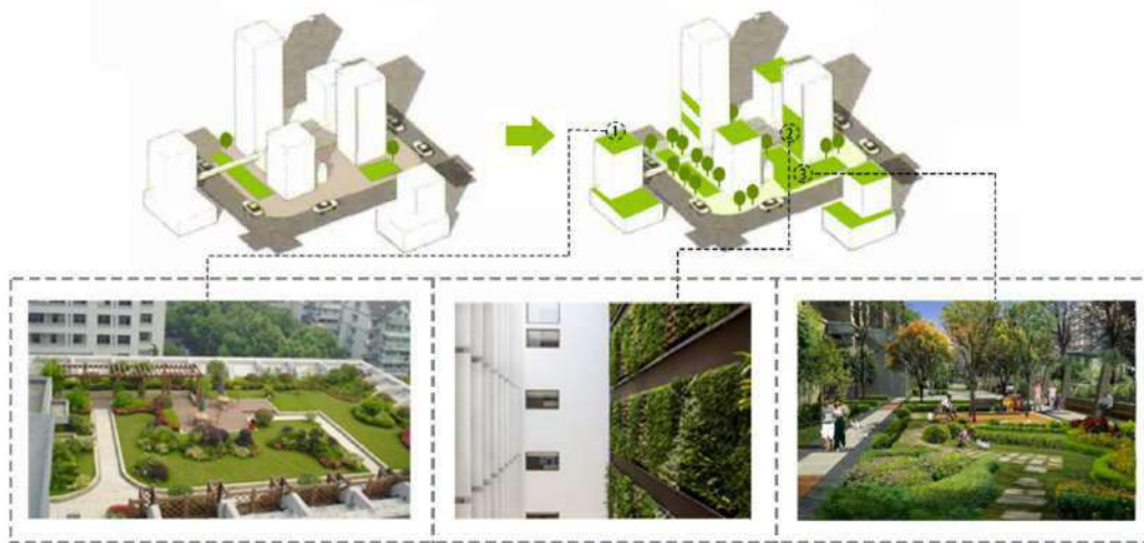
Figure 1: Layout of three-dimensional sponge facilities in old districts Figure sources: drawn by author.
