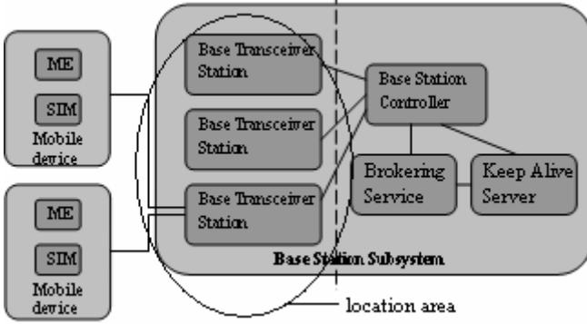
Fig. 1. Proposed Wireless Computational Grid Architecture
