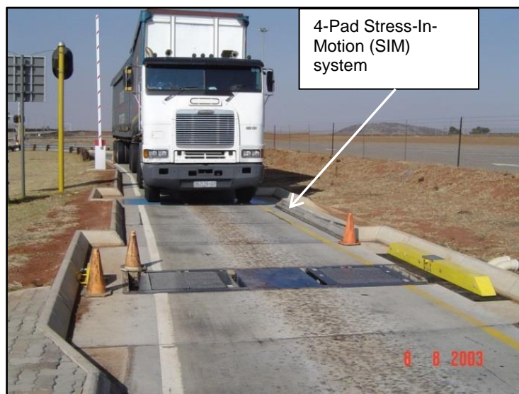
Figure 2. Example of a truck diverted from N3 Freeway near Heidelberg (Gauteng, South Africa) over the experimental site for Stress-In-Motion measurements for each tyre
