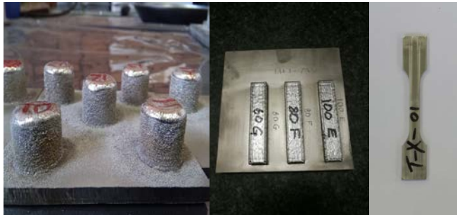
Figure 1 Fabricated Ti-6Al-4V ELI sample coupons and tensile specimen
