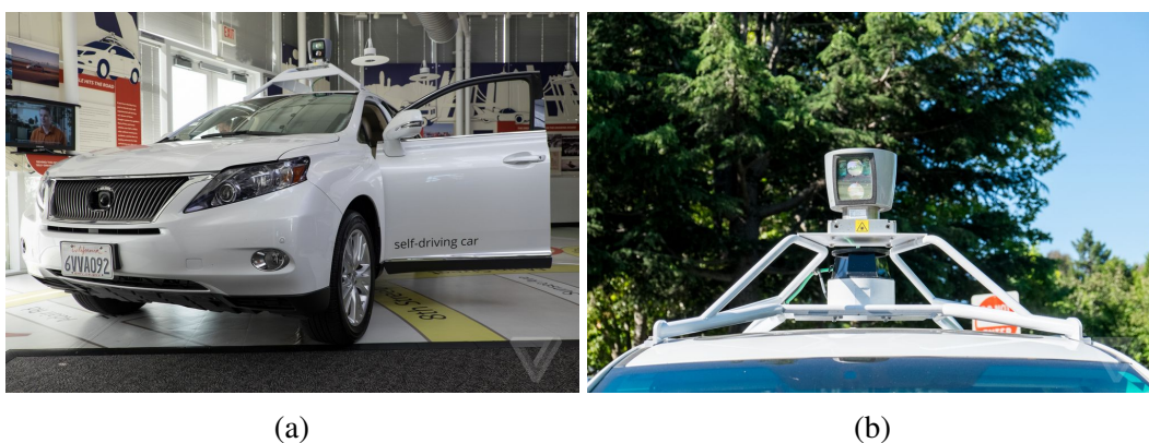
Fig. 1.13 Google's self-driving car (a), with Velodyne HDL-64E S2 LiDAR system (b) [5]
