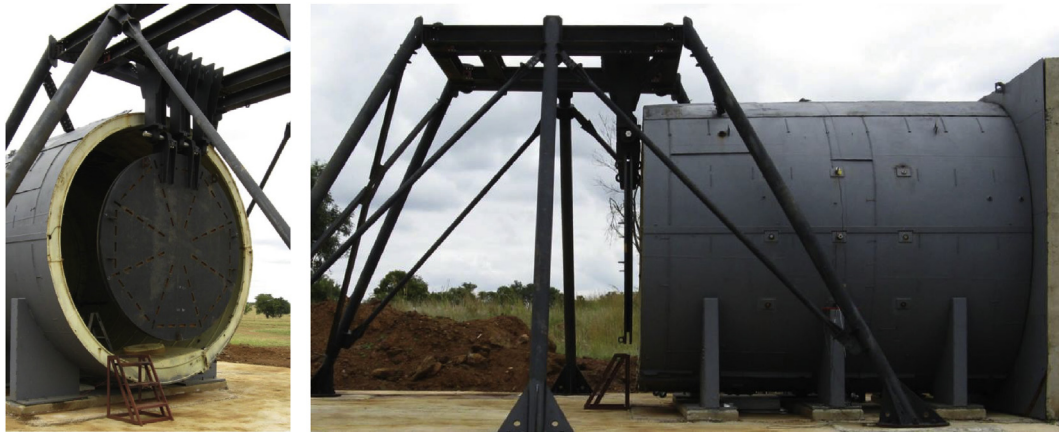
Fig. 8. 5-Ton compound pendulum fitted to the open end of the semi-confined blast chamber.
