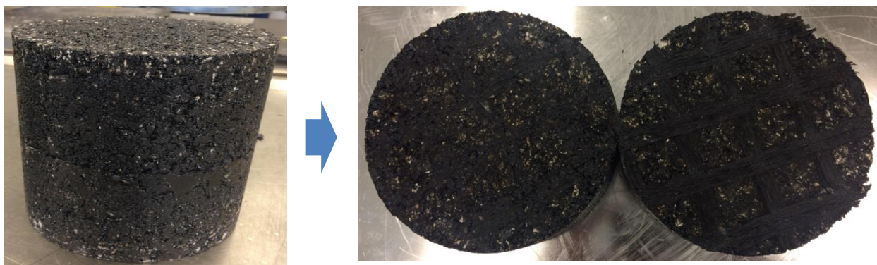
23 FIGURE 6 Example HMA Sample Failure Mode (FA-50 Reinforced).
