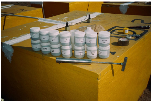
Photograph 4. Coring device and sample bottles
