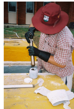
Photograph 5. Expressing cored material into the bottle
