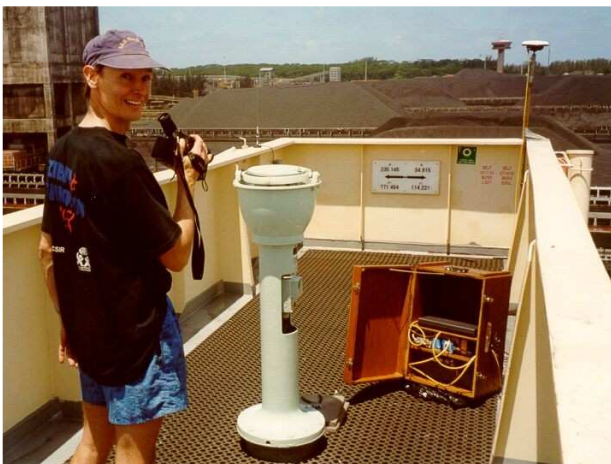
Figure 2: Placement of GPS sensor and computer on board a ship
