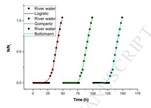
**Fig. 6.** Breakthrough curves of bacterial inactivation using Cts-Bent composites with river water, at a fixed mass load and flow rate of 15 g and 5 mL/min respectively.
