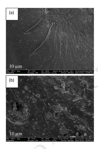
Fig. 1. SEM micrographs of (a) chitosan and (b) Cts-Bent composites.
