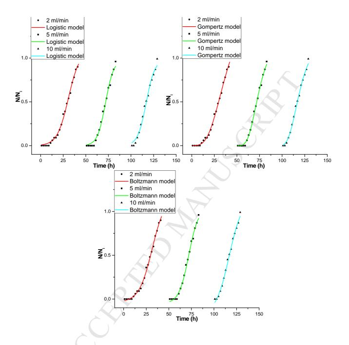
**Fig. 4.** Breakthrough curves of *E. coli* inactivation using chitosan composites with varying flow rates of 2, 5, and 10 mL/min and fixed initial bacterial concentration and bed mass of 5  $\times$  10<sup>3</sup> cfu/mL and 15 g respectively.
