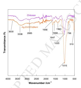
Fig. 2. FTIR spectra of chitosan and chitosan-Bentonite composites.
