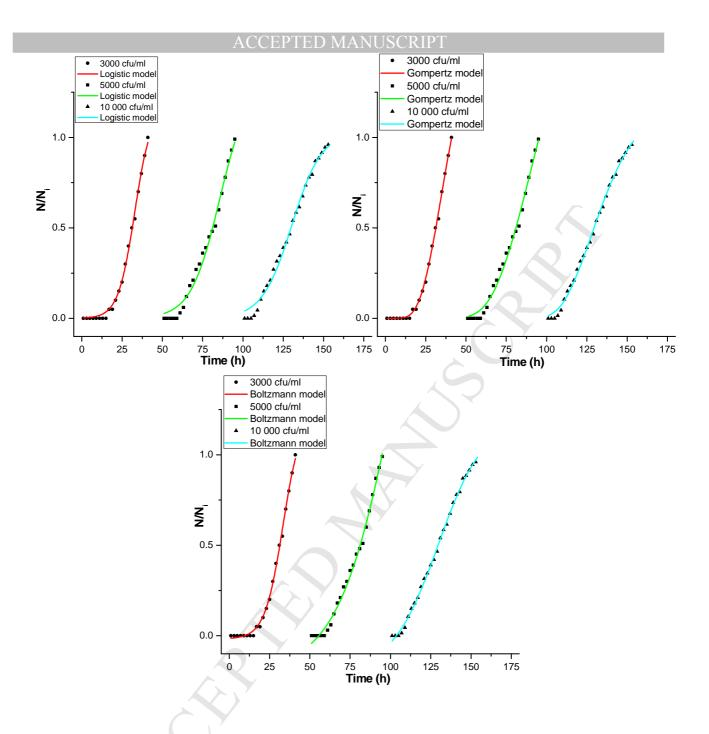
**Fig. 5.** Breakthrough curves of *E. coli* inactivation using Cts-Bent composites with varying initial bacterial concentrations of  $3 \times 10^3$ ,  $5 \times 10^3$ , and  $1 \times 10^4$  cfu/mL and fixed bed mass and flow rate of 15 g and 5 mL/min respectively.
