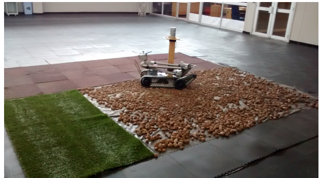
Fig. 1. The layout of the terrain surfaces and the Packbot 510 used for the experiments. The top part is the carpet, grass and rocks are on the sides, while the surrounding area is the rubber.
